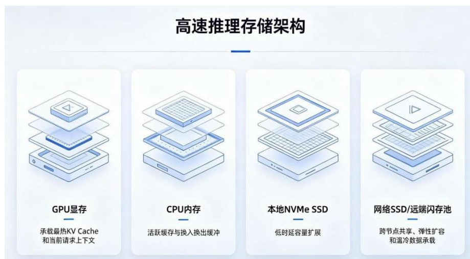
Figure 2.31 Four-tier high-speed inference storage architecture schematic
