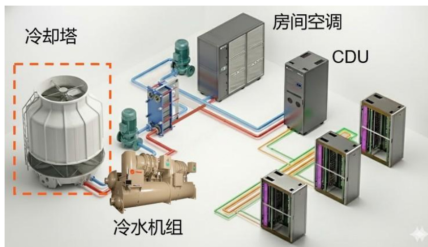
Figure 1.8 Cold-source solution: water-cooled chiller
