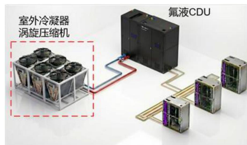
Figure 1.7 Cold-source solution: air-cooled condenser
