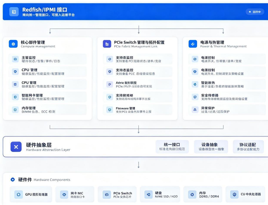
Figure 4.3 Node-level management block diagram
